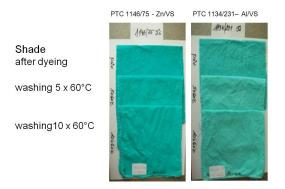
Figure 3: Phthalocyanine dyed cotton fabric (PTC 1146/75 – Zn/VS and PTC 1134/231- AI/VS)
